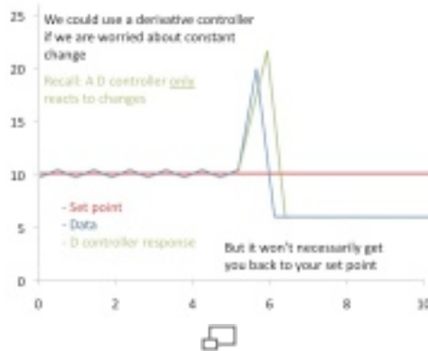
Figure 9. D-controller effect on data.
